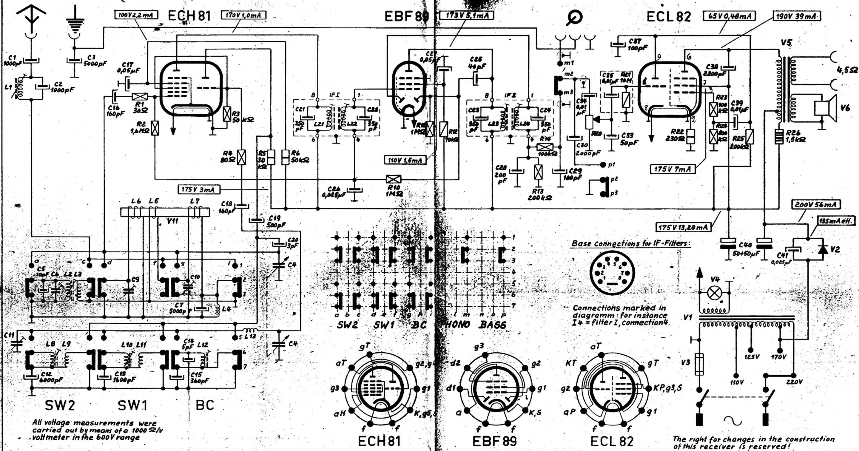
All voltage measurements were carried out by means of a 1000 Ω/V voltmeter in the 600V range
